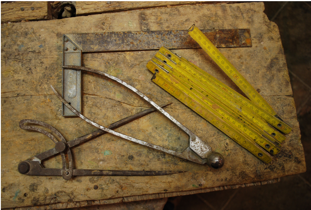
Figure 26: Two varieties of callipers, a set square and a ruler (photograph: B. Russell)
