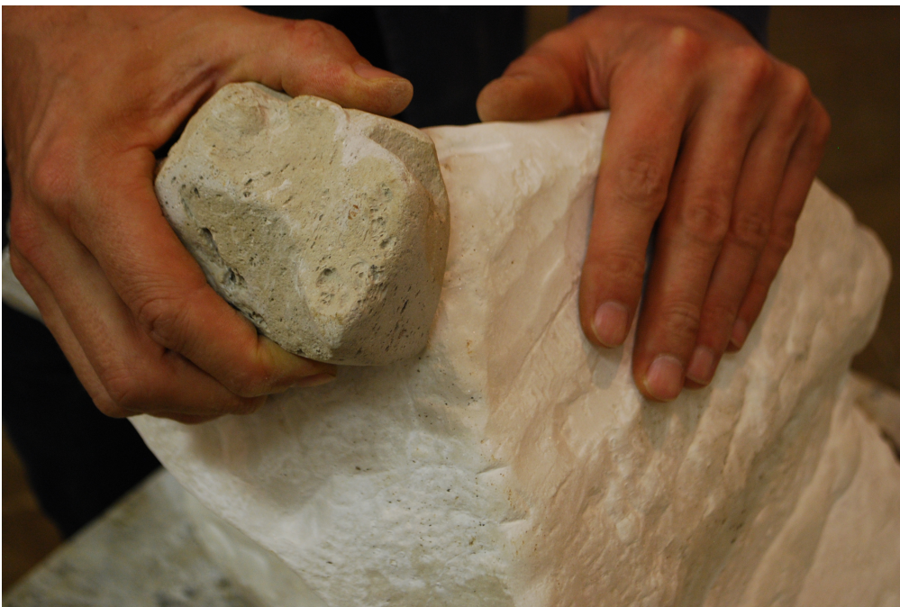
Figure 25: Pumice in use as an abrasive on white marble (photograph: B. Russell)
