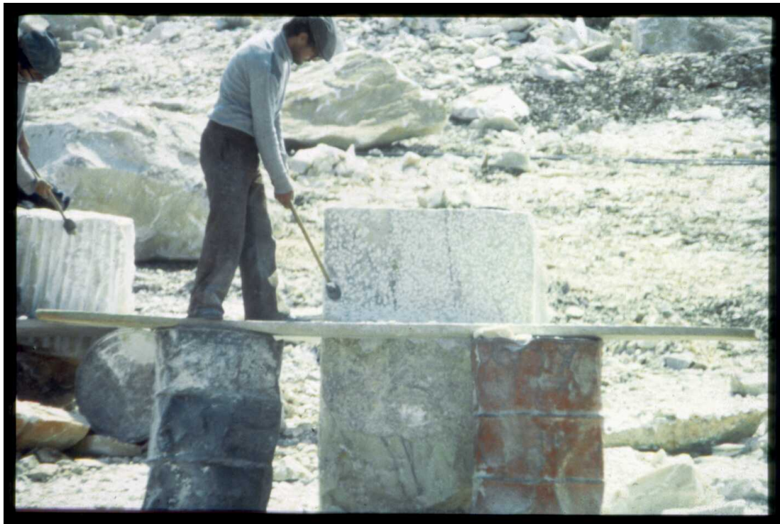
Figure 2: PR936_01_23: Quarryman using a pick to square a block at Iscehisar (ancient Dokimeion)
