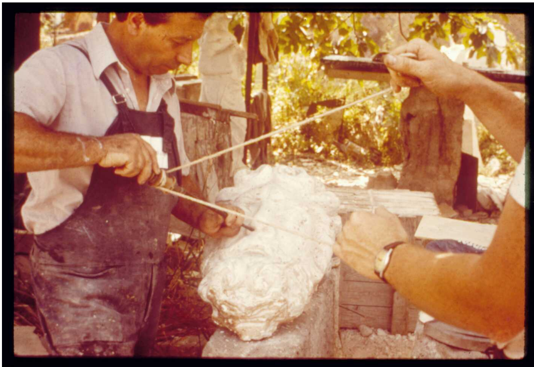
Figure 20: TE_2_1_1_2: Pair of carvers operating a cord drill in the De Tomassi workshop, Rome
